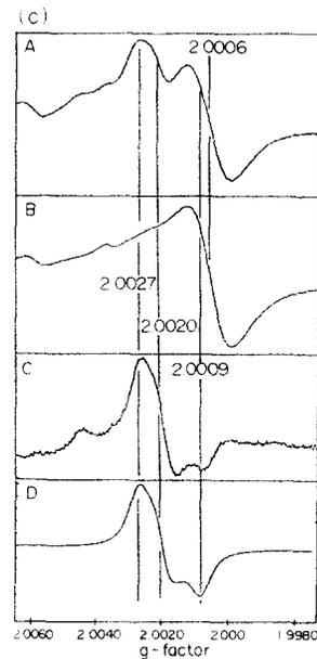
FIG. 5c. Directly after irradiation (A) in foraminifera, a signal superimposes the dating signal at  $g = 2.0006$  which has probably orthorhombic symmetry ( $g$ -factors: 2.0029, 2.0021, 2.0010). It disappears rapidly (B) after gentle heating (90°C). (C) The difference between A and B is due to the unstable signal; (D) computer-simulation of C.
