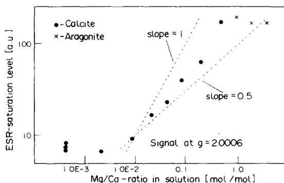
FIG. 7. Saturation level (equivalent for the number of traps) of the signal at  $g = 2.0006$  as a function of the Mg/Ca ratio of synthetic carbonates, grown with a gel-diffusion method (Barabas *et al.*, 1989) (double-log-scale!). The signal amplitude increases by a factor of about 25.
