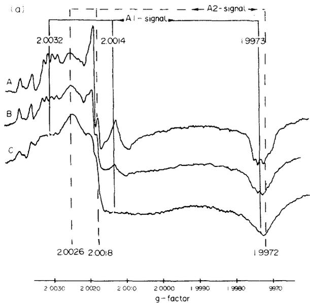
FIG. 5a. Composition of the 'A-signal complex' as derived from annealing experiments: (A) annealed and re-irradiated; (B) plus annealing 2hr/160°C; (C) 5hr/160°C. The 'A1-signal' is less stable and disappears due to heating.
