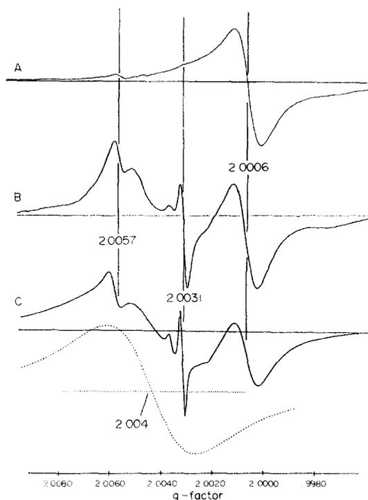
FIG. 6. Examples for natural Mg-calcite with a large signal at  $g = 2.0006$ : (A) red algae, (B) prickles of a sea-urchin; irradiation dose: 500 Gy; microwave power: 20 mW, (C) simulation of (B) (dotted: broad signal at  $g = 2.004$ ).
